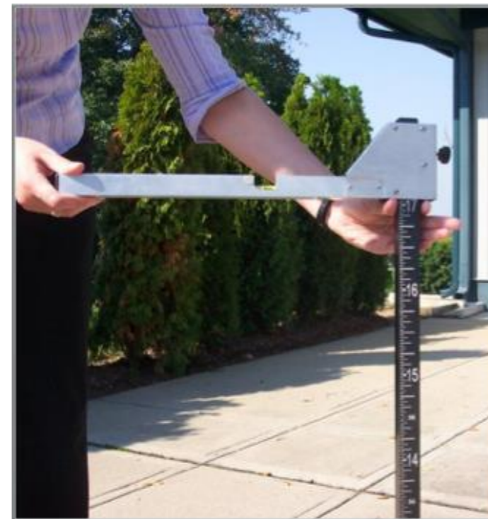
Align the cross arm at top of scale staff
