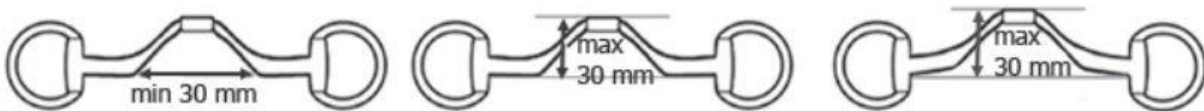
Figure 121.2: Measurement of tongue relief for a snaffle bit. The widest part of the deviation must be where the mouthpiece contacts the tongue and must have a minimum width of 30 mm (left). The maximum height of the deviation is 30mm from the lowest part of tongue side to the highest part of the deviation (center and right).
