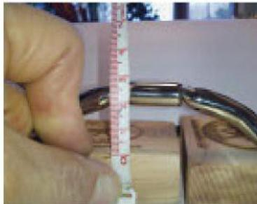
Measurement of a saffle bit to allow tongue relief. The maximum height of the deviation is 30 mm from the lower part of the tongue side to the highest part of the deviation. The widest part of the deviation must be where the mouthpiece contacts the tongue and must have a minimum width of 30 mm.
